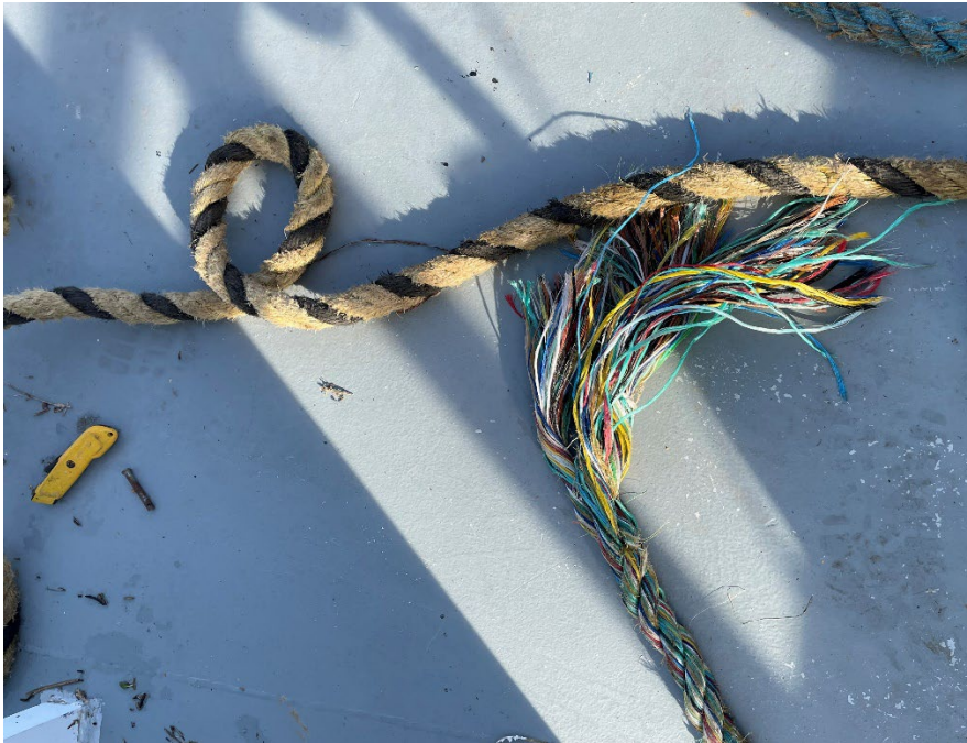
Figure 7. Broken deck line from the WICKLIFFE CREWBOAT used to tie the vessels on the day of the incident. Taken on 3/29/2022 by the Coast Guard at Wickliffe, KY.
